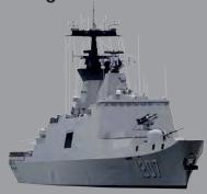
It is responsible for sea frontier defense and joint surface interdiction operations. Capable of carrying out air defense, anti-submarine, escort and anti-blockade operations, it has a stealth hull design that avoids complex shapes and angles, achieving a stealth effect by reducing the reflection of radar waves.
