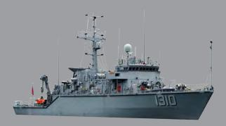
It is responsible for anti-blockade and mine hunting operations. Made wholly of fiberglass, it is not magnetic, with low radar cross section and low cruising noise. Equipped with a mine disposal equipment (unmanned vehicle), it can detect and clear various types of mine.
