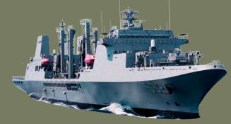
It is responsible for resupply of fuel and ammunition and material transportation. As a mobile sea replenishment vessel, it can simultaneously replenish one ship on either side while cruising. It also has a pair of cranes on the bow deck and amidships, respectively, that are used to load and unload cargo.
