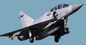
It is responsible for high-altitude interception. The aircraft configuration comprises a large delta wing without tail, and a single engine. It is equipped with two 30mm cannons and carries air-to-air missiles for high-altitude interception operations.
