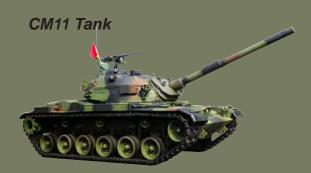
It is responsible for supporting infantry and anti-landing operations. Its main gun has a 2D stabilizer and it is equipped with a new type of fire control system, laser rangefinder, and thermal imager. The CM11 is a main battle tank that can fire when moving and has night combat capability.
