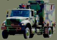
It is responsible for local field air defense early warning and fire allocation missions. It comprises "phased array radar" and "engagement control" sub-systems and can undertake surveillance and tracking against fixed- & rotor-wing aircraft. It can detect enemy targets, provide early warning and prioritize them based on threat levels, increasing engagement preparation time and integrated field air defense effectiveness.
